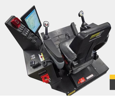
Operational touch panel simulating the interface for the Centurion 5 shovel control system.
