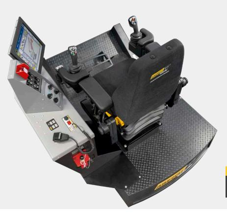
High Fidelity LCD Operator Interface: Operational touch panel simulating the interface for the Centurion 5 shovel control system.
