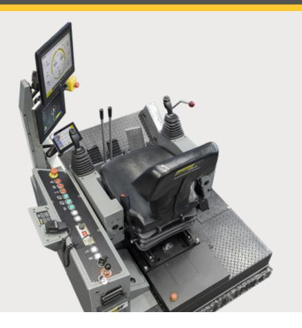
Emulated OEM Machine Control System featuring 15" touch screen, provides exact replication of the real machine enabling operator familiarization and training with the latest OEM interface.
