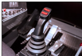
Right hand joystick with truck counter & idle speed switch
