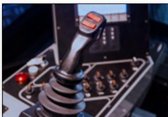
Left hand joystick with swing speed switch & horn
