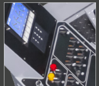
Conversion Kits utilize genuine Komatsu cab controls and instrumentation
