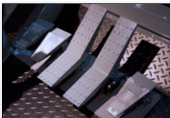
Left & Right propel pedals as well as bucket open & close
