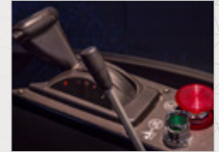
Gear selector, emergency shutdown and fault reset switch
